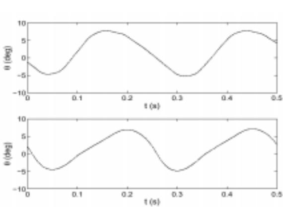
Figure 7: Body angle. Experiment (top), simulation (bottom)
