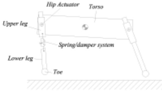
**Figure 3. Scout II mechanical system**
