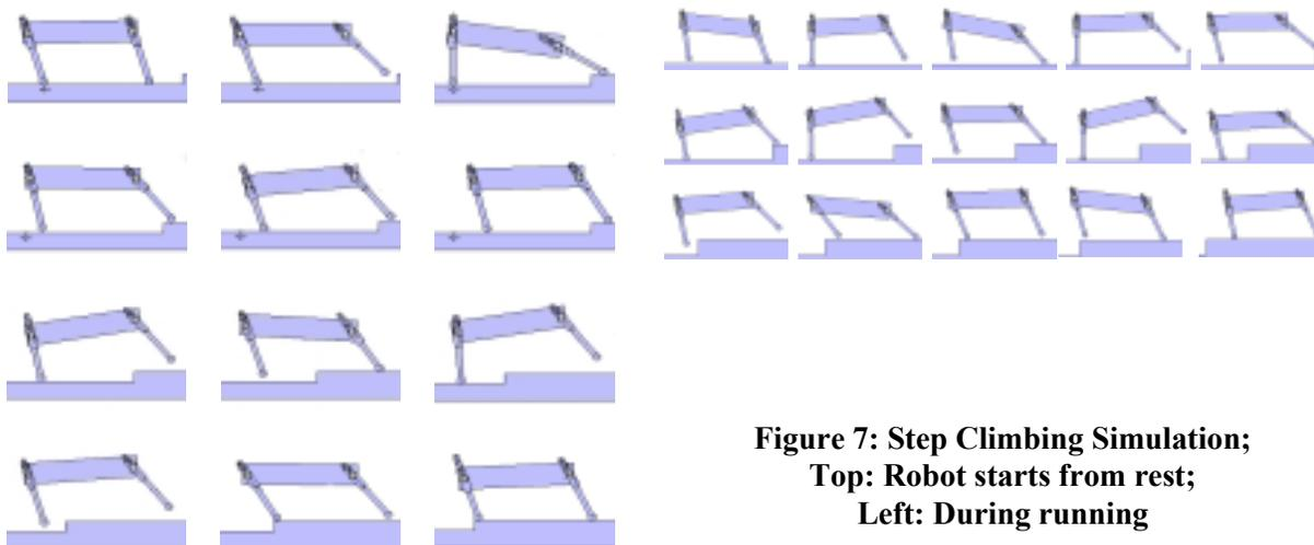
Figure 7: Step Climbing Simulation;
