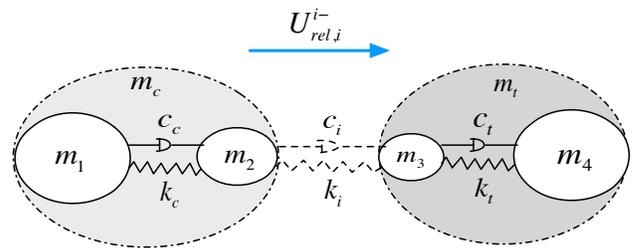
**Figure 2.** Concept for Multibody Contact Model.
