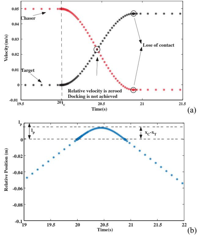
**Figure 8.** Docking Unsuccessful: (a) Velocities of the two bodies before and after impact and (b) Relative position of probe/latch mechanisms in contrast to the required for docking.
