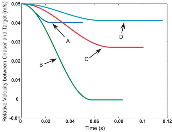
**Figure 7.** Relative velocities between Chaser and Target after first impact. Examples A-D.
