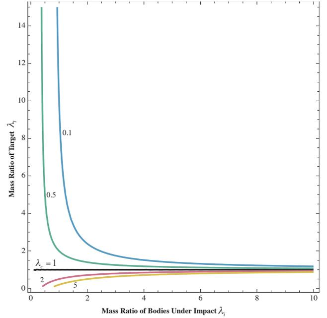
**Figure 5.** Mass ratio combinations which zero relative velocity after impact if the mass ratio of Chaser is known.
