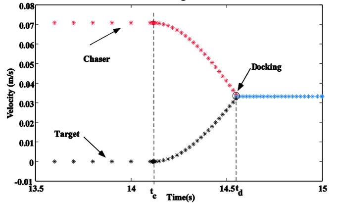
**Figure 9.** Docking Successful: Velocities of the two bodies before and after impact.
