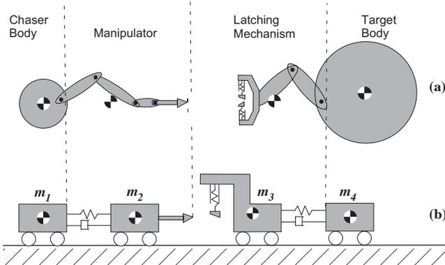
**Figure 1.** Model rationale of impact docking between multibody systems.
