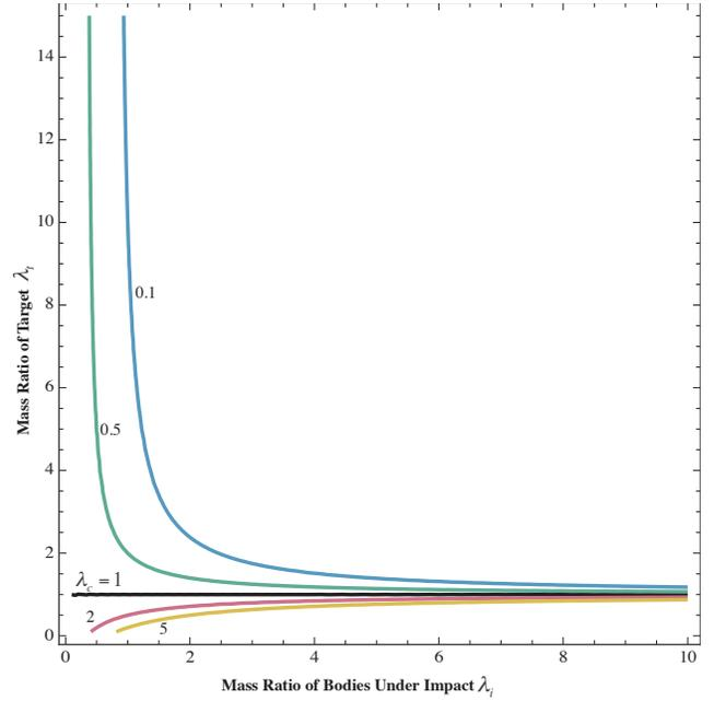
**Figure 5.** Mass ratio combinations which zero relative velocity after impact if the mass ratio of Chaser is known.
