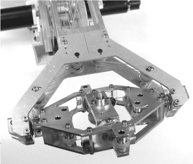
Fig. 7. Assembled spherical joint.
