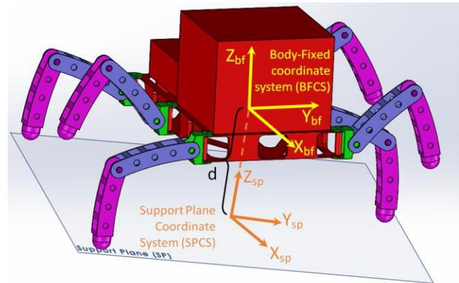
Figure 7. Definition of Support Plane Coordinate System using the Body-Fixed Coordinate System.
