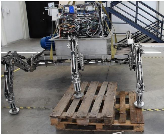
Figure 17. The HexaTerra prototype stepping on multiple objects.
