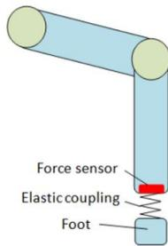
Figure 6. Design of the hexapod foot.
