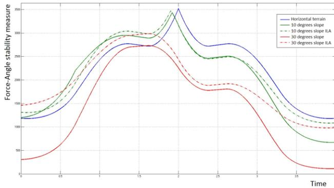
Figure 9. The Force-Angle Stability Measure for moving on slope using typical locomotion algorithm and the inertial locomotion algorithm.
