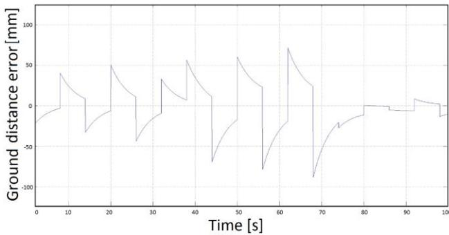
Figure 15. The ground distance error being corrected during hexapod tripod gait in Adams simulation.
