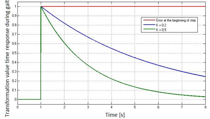
Figure 8.  $z_{err}$ ,  $\text{roll}_{err}$  and  $\text{pitch}_{err}$  error time response with respect to  $K$  gain.
