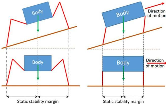
Figure 5. Static stability margin of inertial locomotion algorithm when moving on slope.
