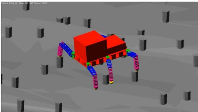
Figure 10. The hexapod stepping on multiple obstacles in Adams simulation.
