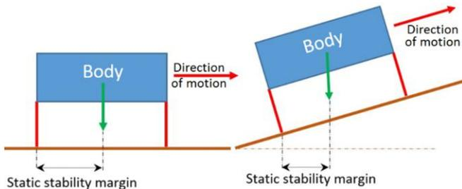
Figure 2. Static stability margin reduction, when moving on a slope.
