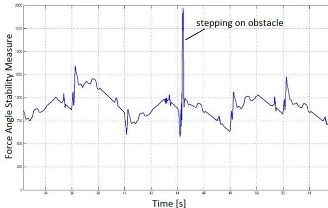
Figure 16. The Force-Angle Stability Measure before and after stepping on obstacle in Adams simulation.
