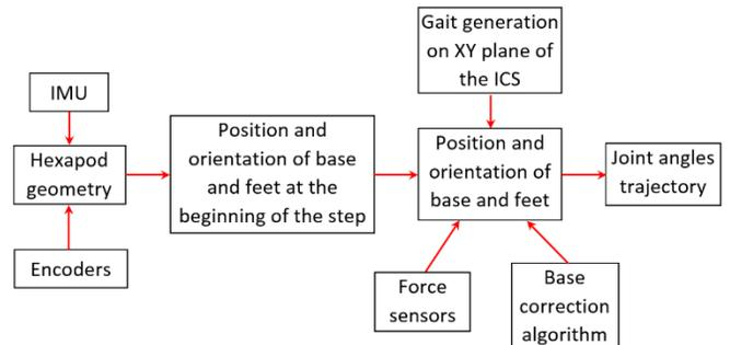
Figure 3. Hexapod locomotion algorithm.
