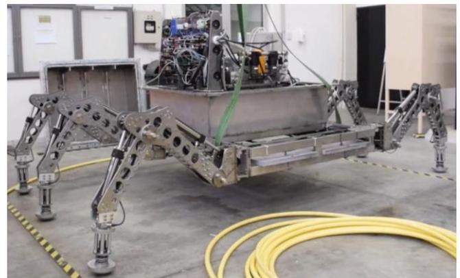
Figure 1. The HexaTerra prototype.
