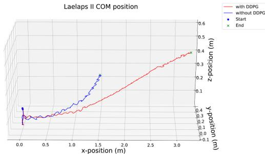
Figure 7. Laelaps CoM while trotting up a ramp of  $10^\circ$ . Without the DDPG layer (blue line), the robot is diverging from its goal and eventually falls. Using the trained policy (red line), the robot manages to reach the end of the 3.2 m ramp.
