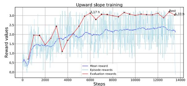
Figure 11. Training and evaluation reward values for inclination of  $+10^\circ$ .
