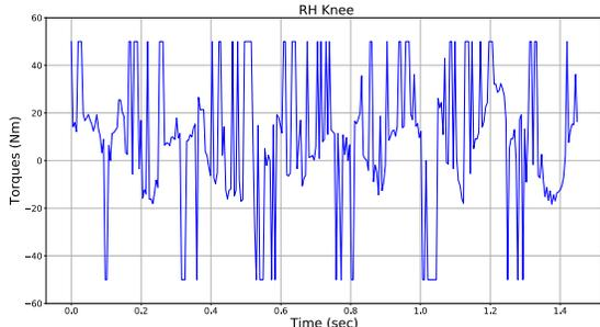
Figure 15. Right hint knee motor torques while Laelaps is trotting up a ramp of  $10^\circ$ . Torques are limited to 50Nm, the same limit that the real Laelaps knee motors are subject to.
