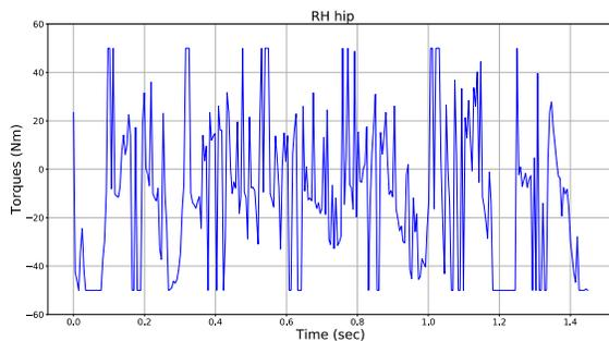
Figure 14. Right hint hip motor torques while Laelaps is trotting up a ramp of  $10^\circ$ . Torques are limited to 50Nm, the same limit that the real Laelaps hip motors are subject to.
