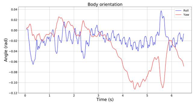
Figure 9. Roll and yaw angles of the Laelaps robot as it is trotting up a ramp of  $10^\circ$  *with* the developed control scheme. The values are bounded for the entire experiment.
