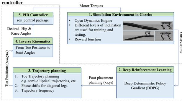
Figure 4. Architecture of the control algorithm.
