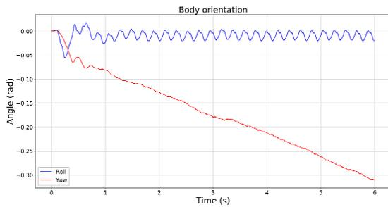
Figure 6. Application of a controller similar to [23] on the Laelaps II 3D model in Gazebo *without* the developed control scheme, and on level terrain. The body roll angle is bounded but yaw angle is increasing.
