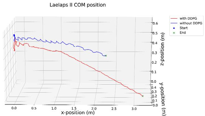
Figure 10. Laelaps CoM position while trotting down a ramp of  $10^\circ$ . Without the developed control scheme, (blue line), the robot is diverging from its goal and eventually falls. Using the trained policy, the robot manages to reach the end of the ramp.
