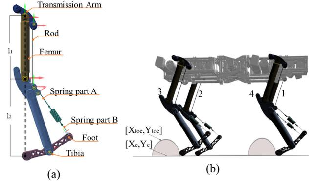
Figure 3. (a) Detailed model of the Laelaps II leg in Gazebo. CAD files were used, and all mass properties were added in the SDF description, (b) Laelaps II Robot in Gazebo. The toes follow semi-elliptical trajectories. Deep RL produces the center of the semi-elliptical trajectories and the trajectory planner produces the exact toe position.
