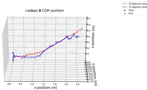
Figure 13. Testing of the learned policy on  $10^\circ$  (red line) and  $15^\circ$  (blue line). In both cases the quadruped reaches the goal.  $10^\circ$  ending point ( $x = 3.18\text{m}$ ,  $y = -0.0078\text{m}$ ,  $z = 0.579\text{m}$ ).  $15^\circ$  ending point ( $x = 3.01\text{m}$ ,  $y = -0.17\text{m}$ ,  $z = 0.68\text{m}$ ).
