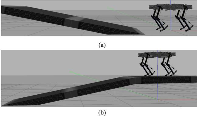
Figure 2. Simulation Environment of Laelaps II Quadruped in Gazebo. (a) Positive and (b) negative slopes are used.
