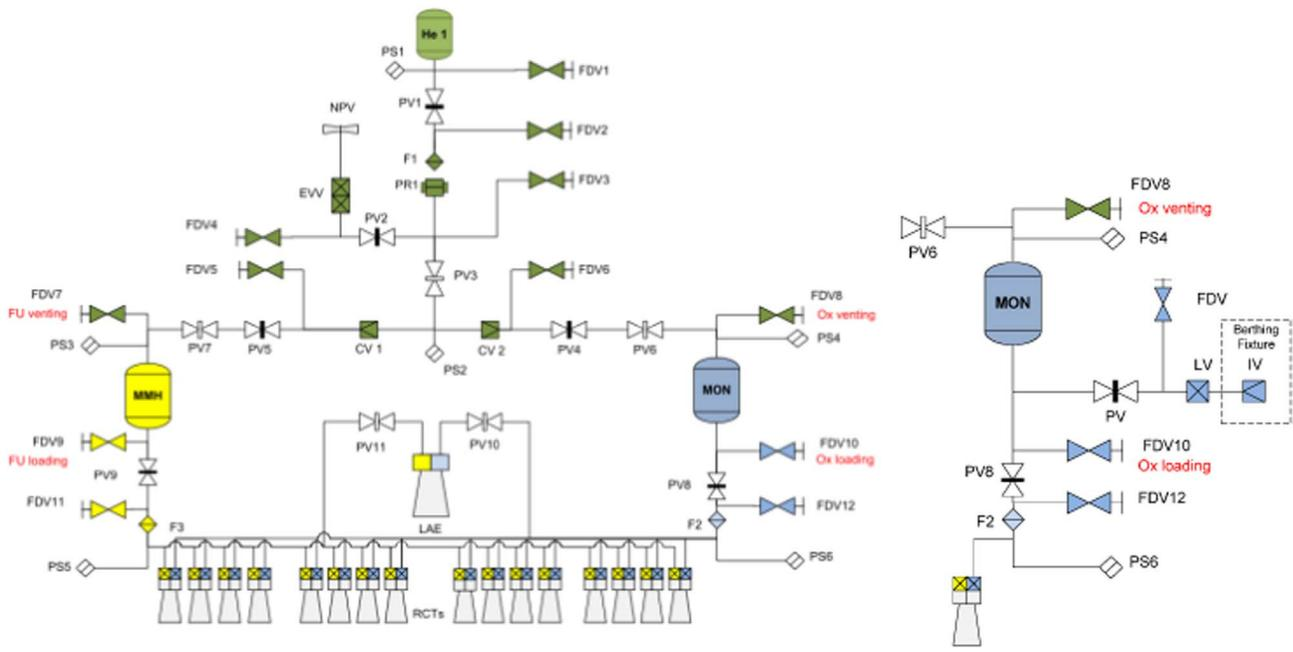
Fig. 7. Generic Bi-propellant propulsion system (left) and MON-refuelling branch (right).
