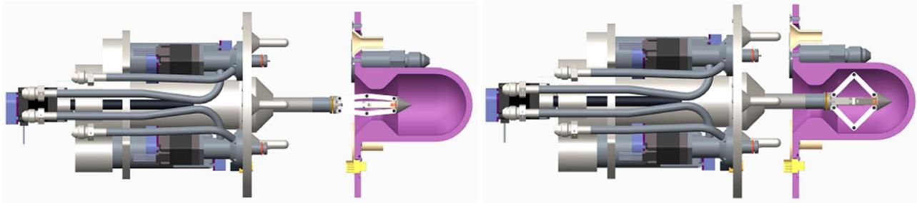
Fig. 4. Pantograph getting introduced into the drogue cavity: initial entrance (left) and deployment (right).
