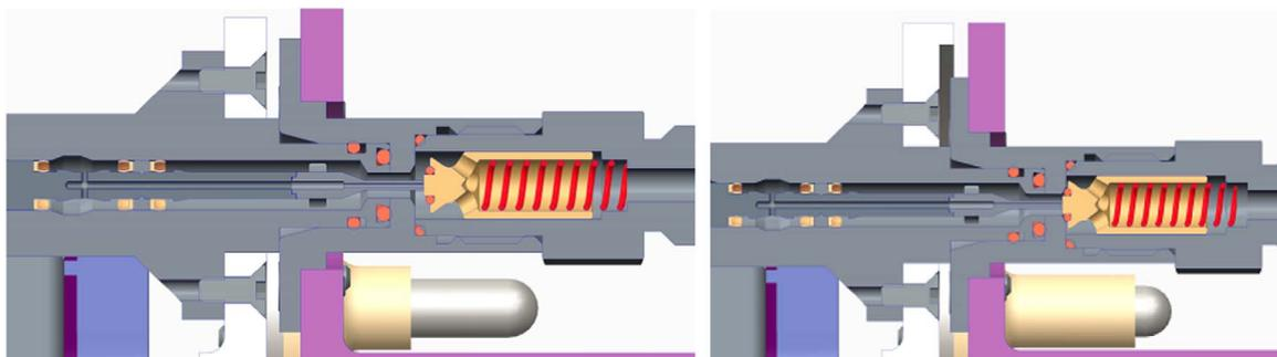
Fig. 6. Actuation valve actuating (left) and releasing (right) the poppet.
