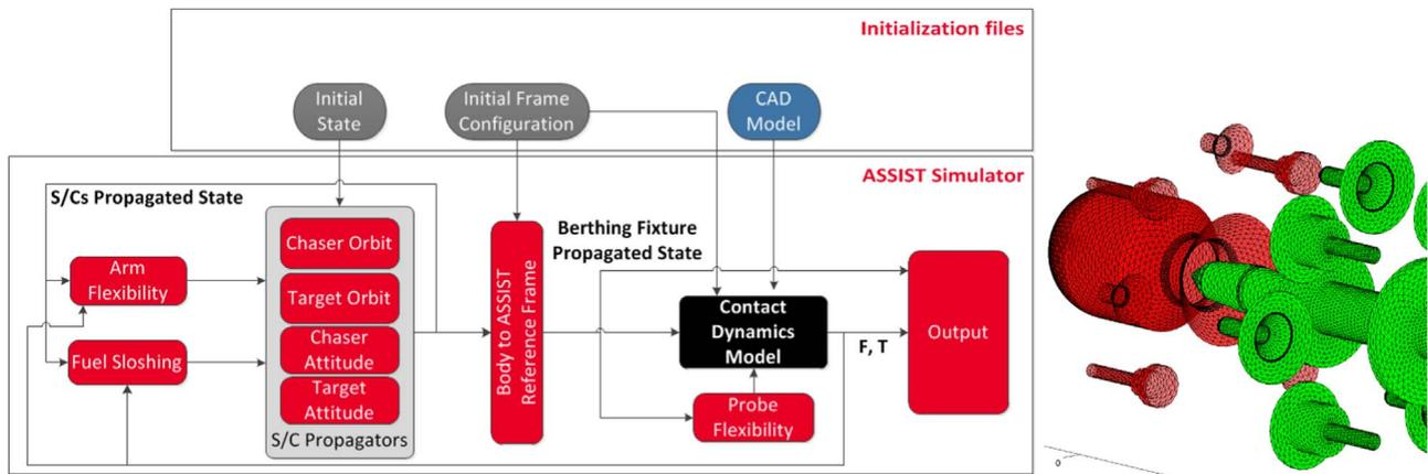
Fig. 9. ASSIST Simulator Architecture (left) and simulation of the docking (right).
