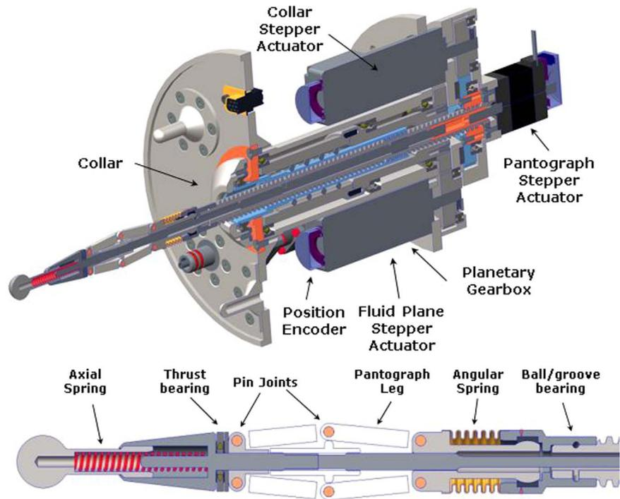
Fig. 2. 3D section of end-effector (top) and detailed probe-tip section with the pantograph mechanism (bottom).
