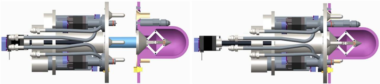
Fig. 5. Pantograph deployed within the drogue: clamping collar attachment (left) and final hard docking (right).
