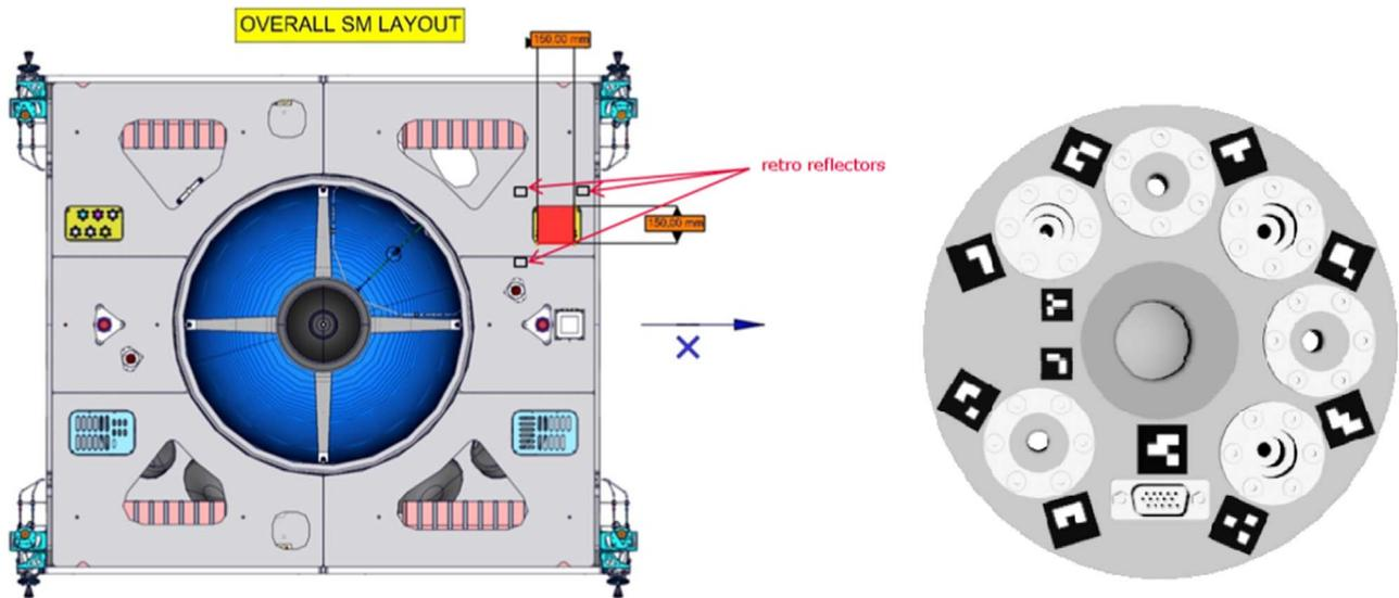
Fig. 8. Example of retro reflectors positioning on the large GEO docking face (left) and visual markers on the berthing fixture (right).
