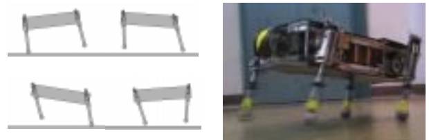
Figure 1: Illustration of a bound gait (left) and Scout II bounding (right).
