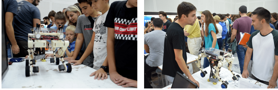
Fig. 6: Maera can be used for short educational events as it is easy to carry and can be controlled wirelessly while a Li-Po battery powers the whole system.
