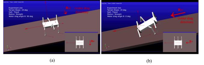
Figure 8. HexaTerra in (a) stable motion ( $\theta = 90^\circ$ ) and (b) tip-over ( $\theta = 0^\circ$ ).
