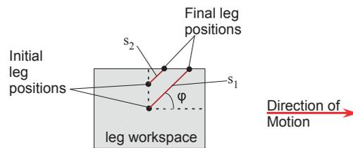
Figure 5. Reduction of the crab and curve motion capabilities when the initial leg positions are extended to the workspace sides.
