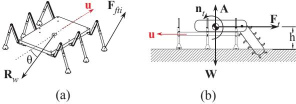
Figure 7. External forces acting on the hexapod robot.
