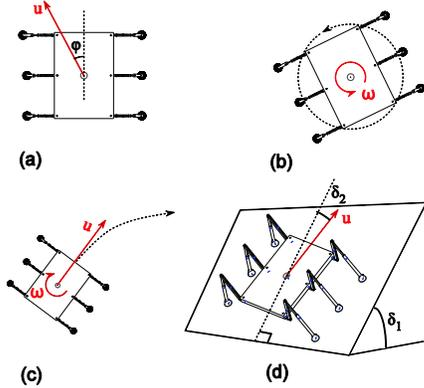
Figure 2. Motion types of the HexaTerra robot: (a) crab motion, (b) pure rotation, (c) motion on a curve and (d) straight motion (on sloped terrain).
