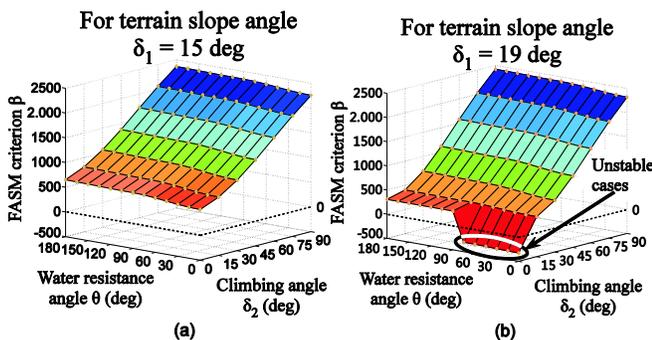
Figure 9. DLSA results for sloped terrain. (a)  $\delta_1 = 15^\circ$  and (b)  $\delta_1 = 19^\circ$ .
