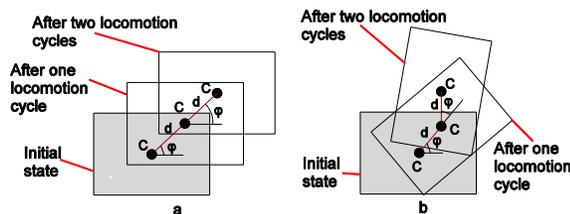
Figure 4. Top-view of the robot base for a) Crab motion, b) Curve motion.
