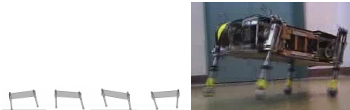
Figure 1: Illustration of a bound gait (left) and Scout II bounding (right)
