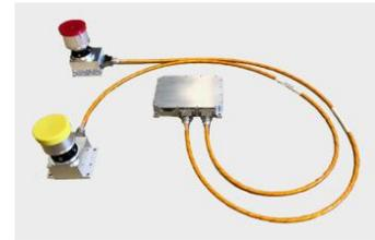
passive sensing in the infrared and visible bands, ARAMIS which stands for Approach and Rendezvous Autonomous Multi-mission Integrated Sensor, is being designed to support all phases of a rendezvous with cooperative and uncooperative targets, from far range to close range and proximity operations.
