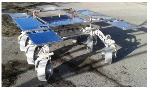
Figure 2.2: Full scale ExoMars type rover integrated by HTR for AWE tests, also equipped with solar panels for outdoor tests.
