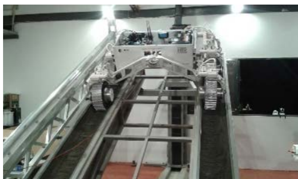
Figure 3.1: Testbed setup for rover tests.
