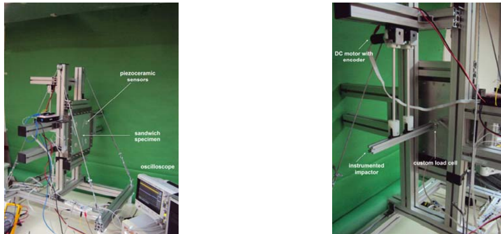
Figure 3: Low-energy impact testing configuration
