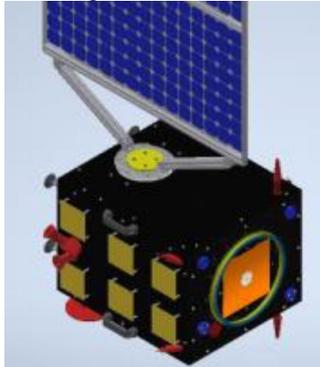
Figure 9 - EROSS Client design in Long-Range configuration for Visual and Thermal Navigation experiments
