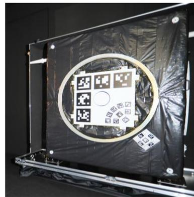
Figure 13 - EROSS Client mock-up in Short-Range configuration
