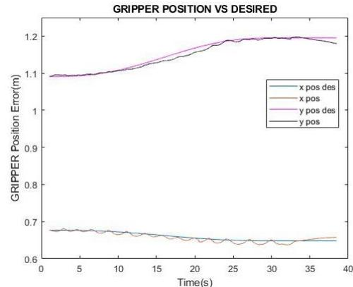
Figure 28 – Gripper reference VS actual position when capturing the Client LAR during the Grasping Test
