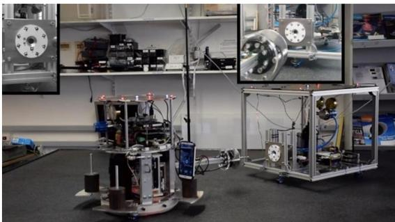
Figure 24 – Chaser robot approaching the Target robot during the ASSIST Dynamic Tests at the NTUA-CSL SRE test bed [ASSIST Project]
