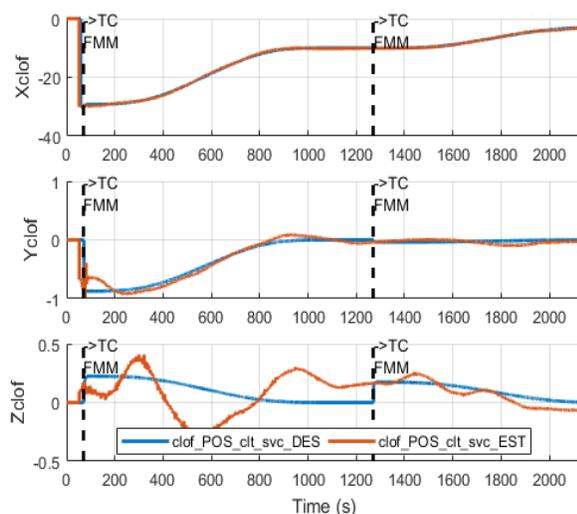
Figure 36 – Desired VS on-board estimate of the relative position of Servicer wrt Client for the **nominal approach**
