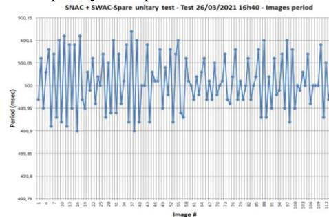
Figure 18 – EROSS SNAC camera unitary test of the acquisition frequency stability over time
