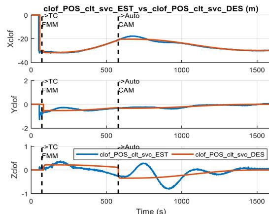
Figure 37 – Desired VS on-board estimate of the relative position of Servicer wrt Client for the **contingency approach**
