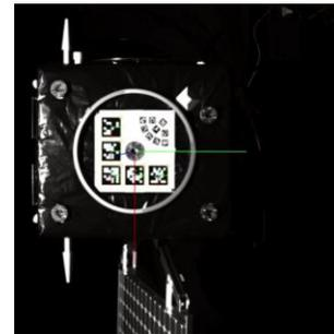
Figure 34 – Marker Tracking using the Visual Camera image running the INFUSE processing solution at short range
