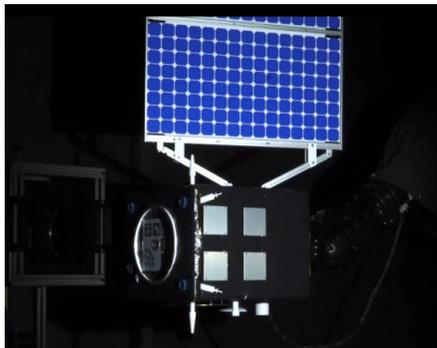
Figure 10 - EROSS Client mock-up in Long-Range configuration
