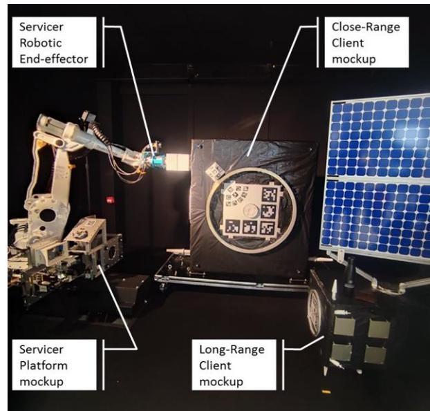
Figure 21 – Autonomy loop setup on ROBY test bench for the demonstration of the ORU exchange service
