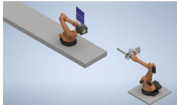
Figure 15 - Long Range Configuration with the Servicer and small Client mock-ups
