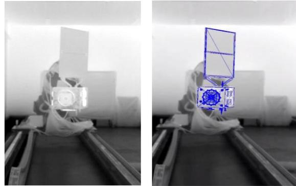
Figure 33 – 3D re-projection on the Thermal Camera image running the ARAMIS processing solution at long range
