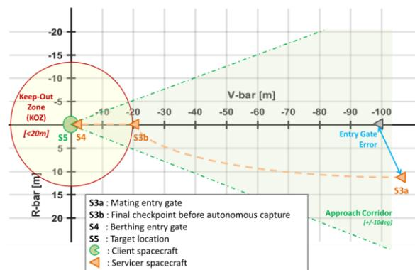
Figure 3 - EROSS final forced motion to approach and capture the Client vehicle
