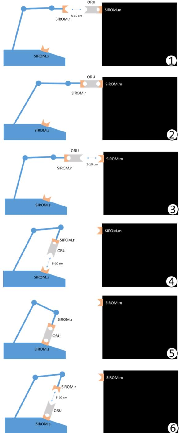
Figure 23 – Steps of the Autonomy loop demonstration with the ORU exchange managed from the RCU and OBC units
