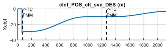
Figure 35 – On-board Guidance profile for the Nominal scenario
