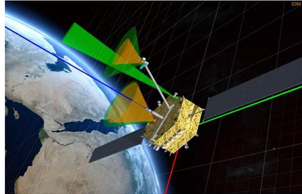
Figure 6 – EROSS Servicer mission design with its robotic arm and rendezvous and robotic sensors Fields-of-View
