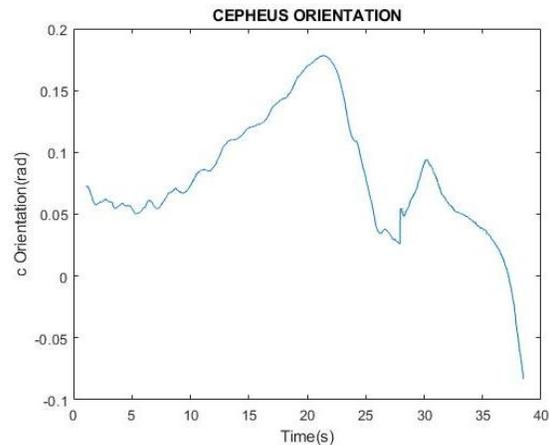
Figure 29 – Servicer base orientation error when capturing the Client LAR during the Grasping Test
