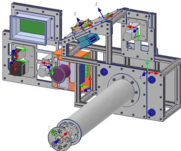
Figure 7 – EROSS Servicer mock-up design with the reference frames of each equipment
