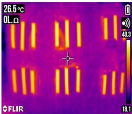
Figure 11 – Squared heaters calibration on the side of the Client Long-Range mock-up
