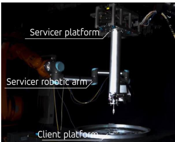
Figure 5 - Illustration of EROSS Servicer and Client mock-ups from the experimental perspective
