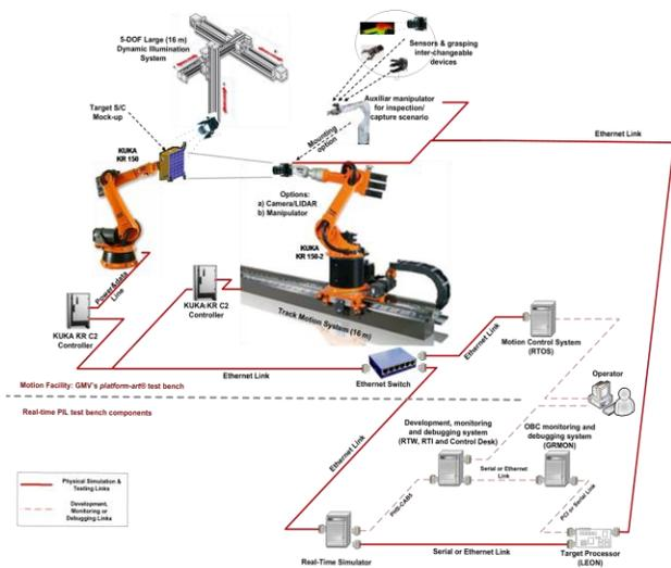
Figure 31 – Platform-art® kinematic test bench architecture (example with a PIL/LEON configuration)
