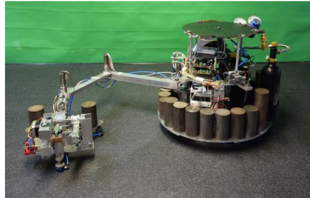
Figure 25 – Free-floating EROSS Servicer mock-up based on the Cepheus vehicle with the gripper functional mock-up
