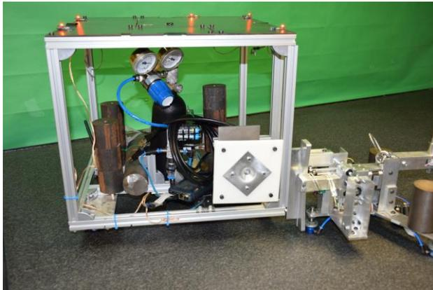
Figure 26 – Free-floating EROSS Client mock-up based on a passive vehicle with the LAR and ASSIST interfaces
