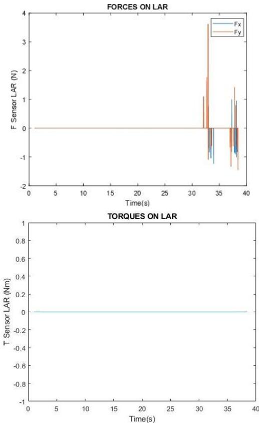
Figure 27 – Resulting Force/Torque measurements at the gripper level when capturing the Client LAR for the EROSS grasping experiment
