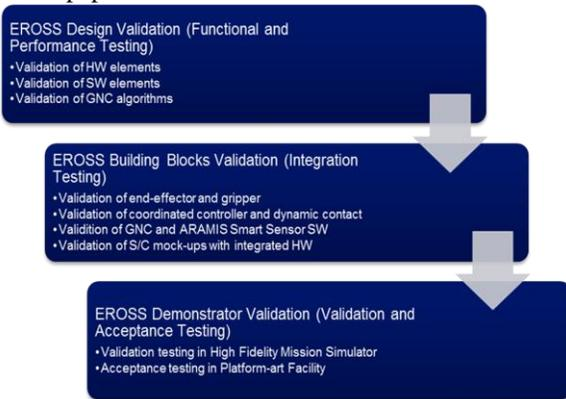
Figure 14 - EROSS Validation Approach with Functional testing, Building Blocks integration, and Validation testing
