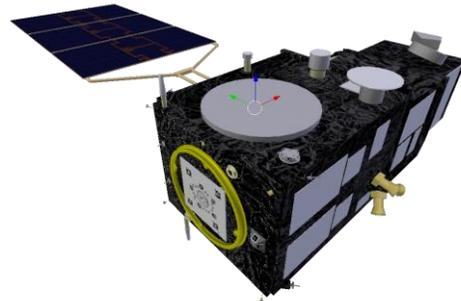
Figure 8 - Illustration of the EROSS Client satellite with markers and refueling/standard interfaces
