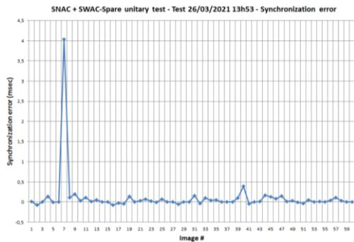
Figure 20 – Time synchronization error between the acquisition of SNAC & SWAC cameras for GNC integration
