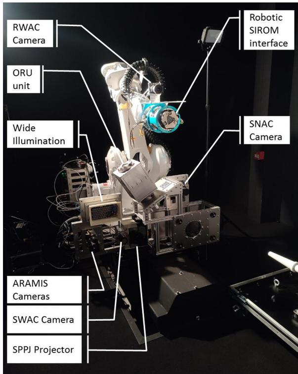
Figure 22 – Servicer Platform & End-effector setup on ROBY test bench for the Autonomy loop demonstration
