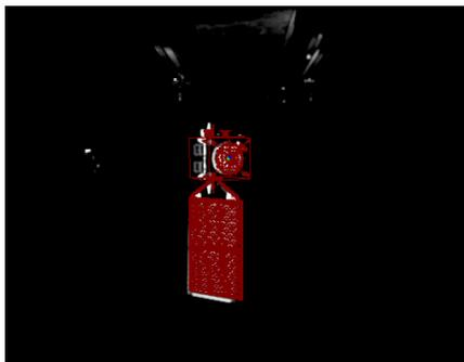
Figure 32 – 3D model re-projection on the Visual Camera image running the INFUSE processing solution at long range
