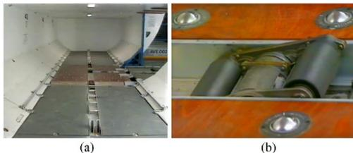
**Fig. 1.** (a) Typical Cargo Compartment. (b) Power transfer units inside the A320 CC.
