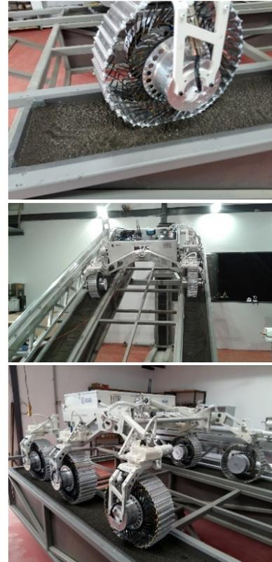
Figure 2: Wheel breadboards testing at HTR Laboratories on single wheel (top) and subsystem level testbeds (middle and bottom) using crushed basalt as soil.
