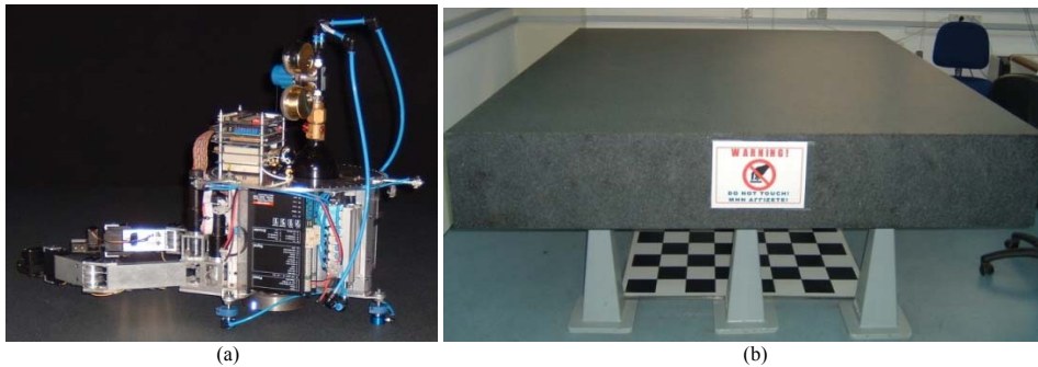
Fig. 2. (a) The robot floating over the granite table, (b) The granite table in the laboratory.
