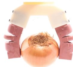
Fig. 1. A prototype soft gripper based on the developed electromagnetic actuator firmly grasps and lifts an onion.
