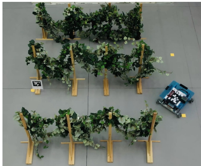
Fig. 1: Drone view of the CSL rover in the synthetic vineyard developed in the lab.
