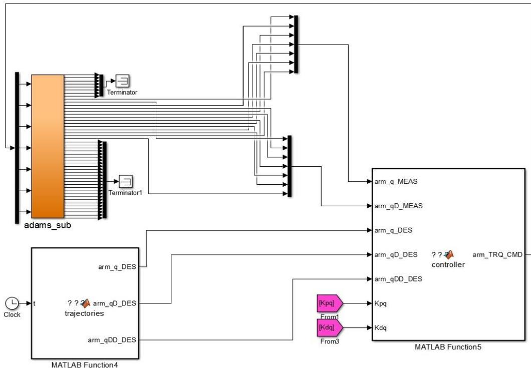
Figure 9: The Matlab/ Simulink model of the AJSC mode.
