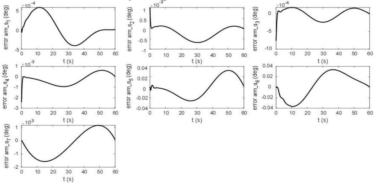
Figure 10: Joint angle errors during the AJSC validation test.
