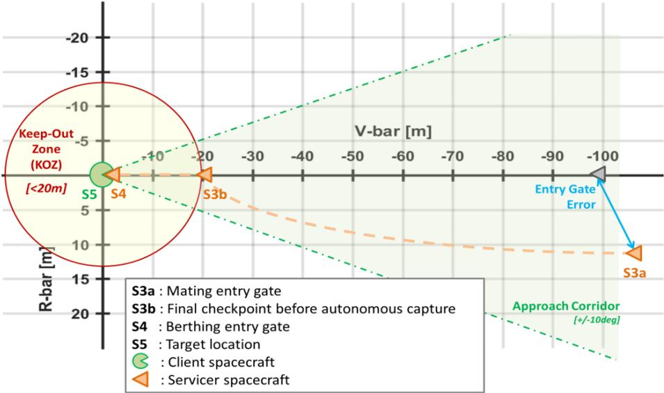
Figure 4: EROSS final forced motion to approach and capture the Client vehicle.
