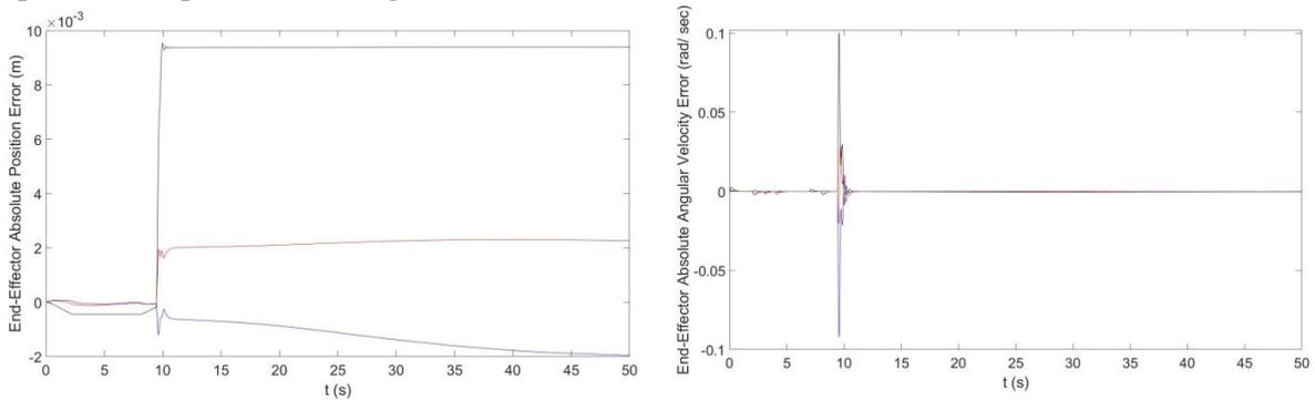
Figure 16: End-Effector position & rate errors during the compliant ICCC validation test.
