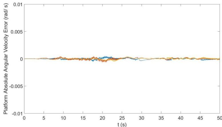
Figure 17: Servicer platform angular velocity during the compliant ICCC validation test.
