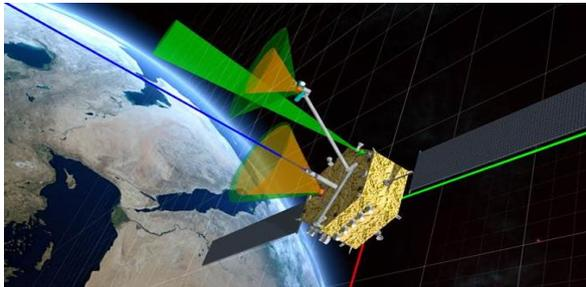
*Figure 6: Rendezvous and robotic sensors FoV with the deployed arm.*
