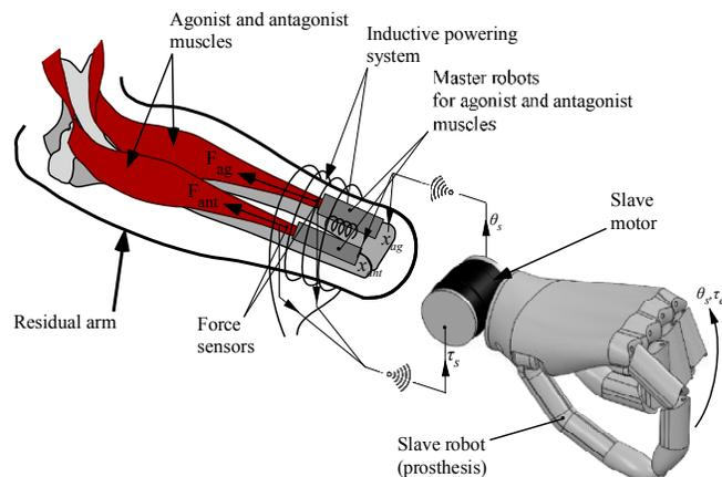
Figure 1. A Biomechatronic prosthetic hand controlled by a wireless Master-Slave teleoperation system [5].
