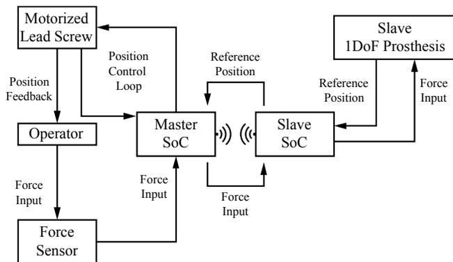
Figure 2. Architecture diagram of the real-time implementation of the Biomechatronic EPP Prosthesis Controller using BLE wireless technology.
