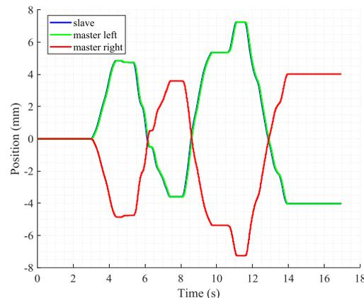
Figure 4. Master motors positions follow Slave motor position response.
