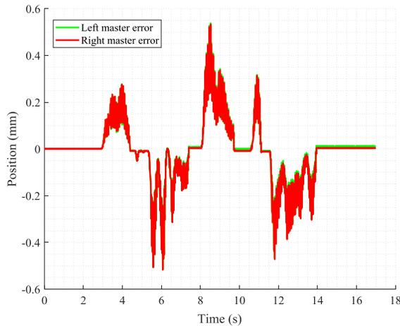
Figure 5. Position error between Master motors and Slave motor.
