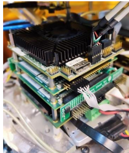
Figure 5. The upgraded PC104 module and the front I/O Cards that send commands to thrusters.
